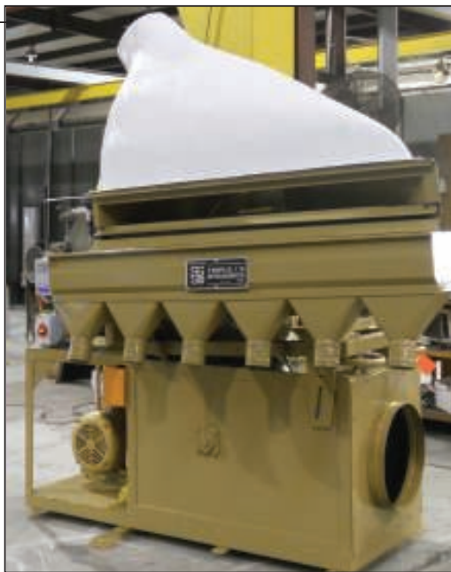
FIGURE 2. Bulk solids are separated and move through gravity-separation machinery based on terminal velocity and gravity
