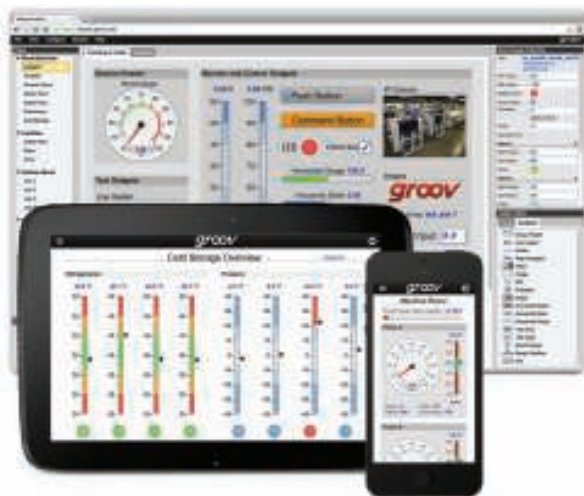
FIGURE 3. The groov, which allows access to a facility's automation system from a mobile device, makes mobile devices more accessible. It allows users to build mobile operator interfaces — customized mobile apps — and securely monitor and control just about any automation system and equipment
