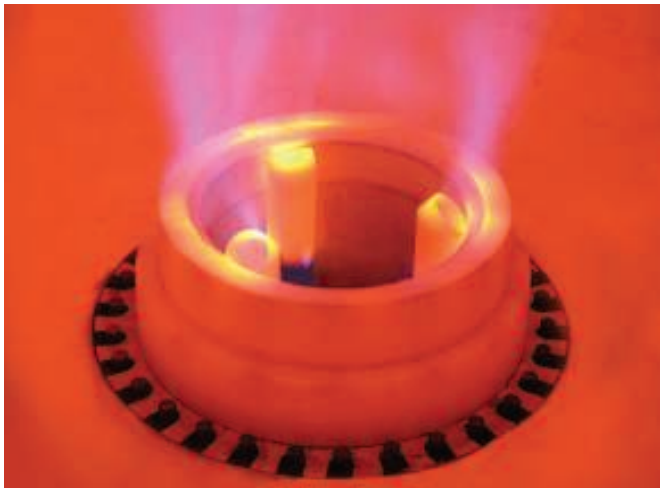
ZEECO® Ultra-Low NOx GLSF Free-Jet Burner
